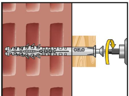
Turn in the special screw with a screwdriver to fix the fixing part.
