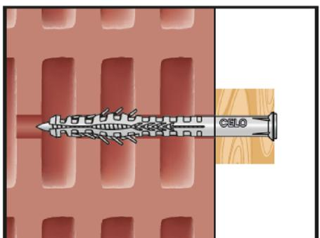
The plug is mounted correctly when the screw is completely in the plug.
