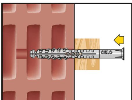
Put the plug completely into the hole. The plug must be long enough that the setting depth is ensured.
