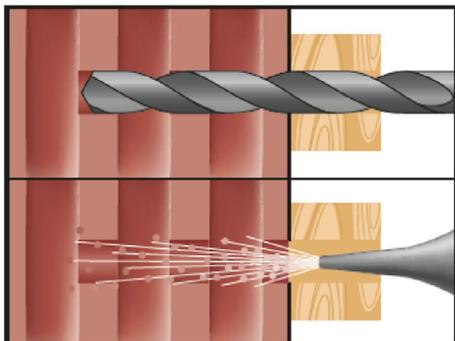
Make the drill hole (can be drilled also through the fixing part).
