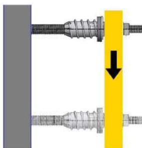
**Maximum shear loads V<sup>1)</sup> at max. 3 or 5 mm displacement per ResiTHERM®
