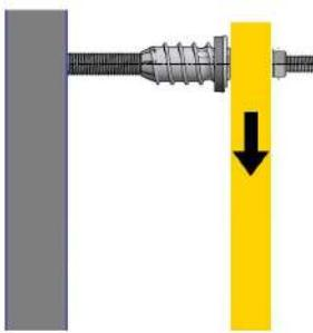
**Maximum shear loads V<sup>1)</sup> at max. 3 or 5 mm displacement per ResiTHERM® if the free outer end of the ResiTHERM® 16 & 12 is freely rotatable at 24°C/40°C<sup>2)</sup>**
