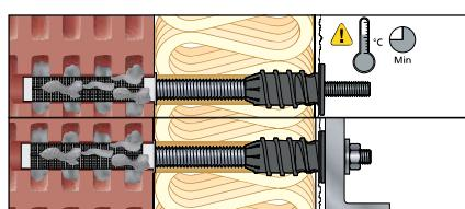
**Note:** The thermal separation module drills itself through the insulation (additional sealing is not necessary, unless the plaster is very rough)
