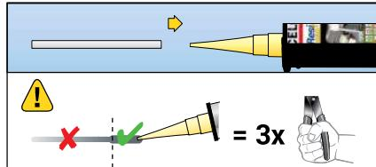
4. Attach the mixing nozzle extension MDV to the mixing nozzle MD. Squeeze out the injection mortar until the mortar has a uniform grey mixing colour - discard the pre-run of the first at least 3 strokes.
