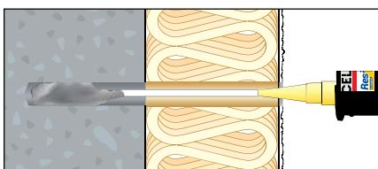
5. Fill at least 2/3 of the drill hole with composite mortar (start from the beginning). For number of strokes see mounting instructions at
