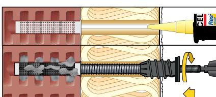
7. Fill the plastic sleeve completely with composite mortar (start from the beginning). For number of strokes see mounting instructions at
